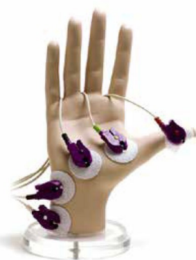
Electromyography (EMG) Requires 5 electrodes
